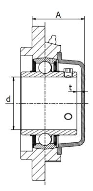
S = Open sheet steel cover SM = Closed sheet steel cover
